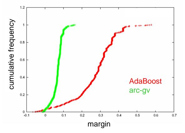
The minimum margin is bigger for arc-gv, but the overall margins distribution is higher for AdaBoost
